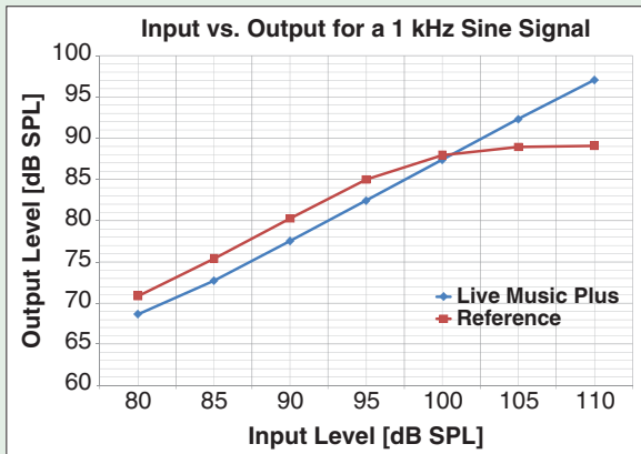
Figure 3. A comparison between the input and output functions with Live Music Processing on and off.
