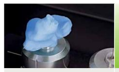
**1.** The process begins with the digital scanning of each client's ear impression, which is stored for future reference in case of a style change or lost custom product.
