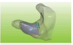
**3.** The optimum placement of components and venting options is then determined, taking into account the individual's anatomy and audiological needs.
