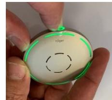
4. To install a RogerDirect receiver code into a Marvel hearing aid, push the pin tool into the button hole farthest from the S/N and hold it there for **2 Sec**
