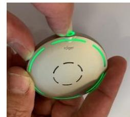
4. Push the pin tool in the button hole farthest from the S/N and hold it there for **2 Sec.**
