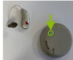
3. The following light indication shows the number of receiver codes available in the iN transmitter e.g. two green flashes = two codes available
