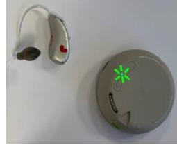
2. Check that there are empty slots available for the receiver code in the Roger Select iN by **briefly** pushing the pin tool into the button hole farthest from the S/N.
