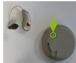
3. The following light indication shows the number of empty slots available in the iN transmitter e.g. one green flash + one red flash = one code + one empty slot available
