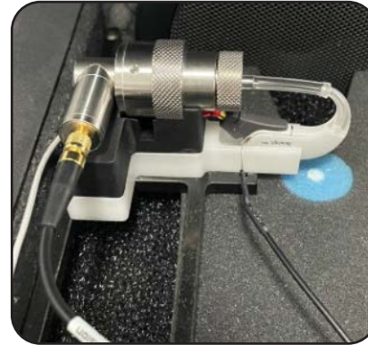
Test jig, DSA7000 attached to the BLK test frame and placed in the ATC400/TBS25 sound chamber
