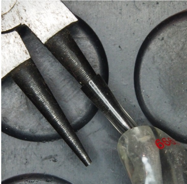
Fig 4a: Enlarging tube for a tight fit, b: Enlarging tube for an even tighter fit
